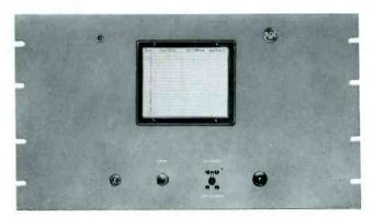
Front view of BTR-20B Transmitter Control Unit.
